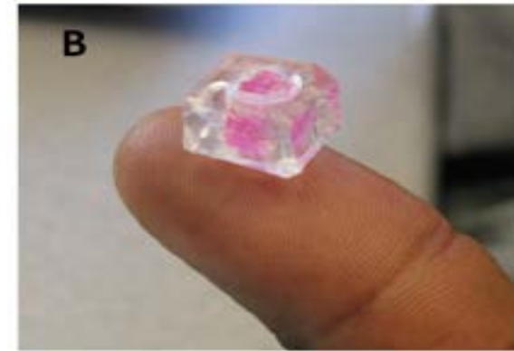
Prototype BioMENS fabricated domestically for use in targeted cancer drug release
