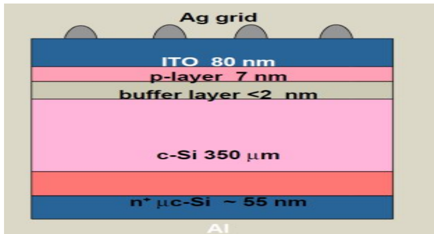
High Efficiency Silicon Heterojunction solar cell developed in collaboration with IMM-CNR Italy
